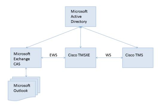
Cisco TMSXE communicates with Exchange or Office 365 using Exchange Web Services (EWS).
